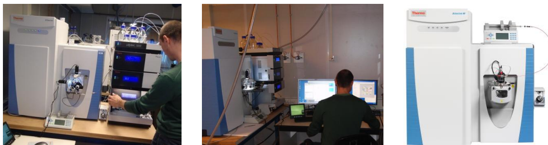
Figure 4. OPL infrastructure consists of 3 nanoLC-MS/MS set-ups (two first generation QExactives and one QExactive HF platform).
